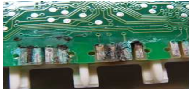
Corrosion Damage Example
